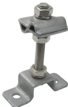
DPK-85GTS is used as part of grounding, lightning protection and potential equalization systems. Designed for fastening (parallel and perpendicular connection) of round clamped conductors (down conductors) to horizontal and vertical surfaces of buildings and structures, including roofing such as: soft roof, corrugated board, metal, sandwich panel. Hot-zinc coated steel in accordance with GOST 9.307-89.
