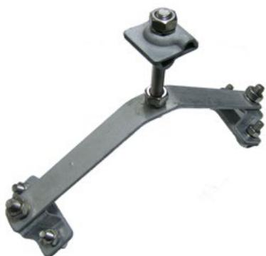
KD-1.1-100-115GTs is used as part of grounding, lightning protection and potential equalization systems. Designed for fastening (parallel and perpendicular connection) of round clamped conductors (down conductors) to the ridge of the roof of buildings and structures, including roofing such as: soft roof, corrugated board, metal, sandwich panel made of combustible and non-combustible materials. Hot-zinc coated steel in accordance with GOST 9.307-89, stainless steel fasteners.
